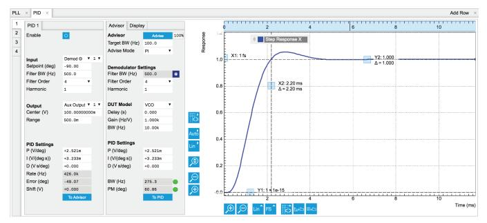
Each of the 4 PID controllers has a dedicated tab with the main controller settings in the left section, the DUT model settings and auto-tune further to the right and a large diagram to see the modelled transfer function or step-response.
