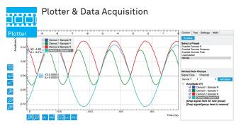
The Plotter and Data Acquisition module display multiple measurement data in the time domain. The Plotter displays the data continuously and the Data Acquisition module captures individual shots based on numerous internal and external trigger conditions.
