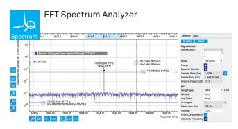
The Spectrum Analyzer takes any of the demodulators' signals or frequency as an input and applies a fast Fourier transform. The main features are:
