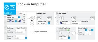
Every demodulator has a graphical representation in the form of a block-diagram for intuitive instrument. In addition, the overview tab allows the control of all demodulators, signal inputs and signal outputs from a single panel.
