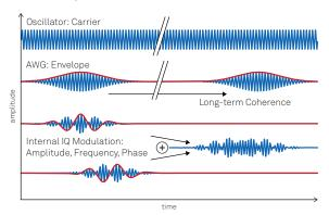
The HDAWG is equipped with digital oscillators to generate the sinusoidal carrier of a signal independently of the programmed AWG envelope signal. This means that long signals can be generated with very fast waveform upload and precise phase coherence across many pulses. Carrier frequencies and phases that would otherwise be written to a static waveform can be freely adjusted and swept.
