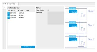
With MDS multiple HDAWGs can be operated much as a single multi-channel AWG:
